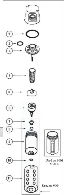
Wash filter element at intervals with naphtha to maintain filtering efficiency. To clean element, depressurize system, unscrew bowl, and unscrew element from head. Dry the filter element thoroughly before reassembling. Clean filter bowl(s) only with soapy water. Inspect O-ring, replacing if damaged or distorted. Reassemble with care to avoid stripping threads on bowl.
